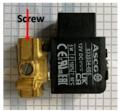
The Manual Override can be used to check that the system is working properly. To test the system manually (eliminating the timer and all electrical), with the air pressure on full (140 psi), turn the screw ¼ turn to horizontal. This opens port 1 to 2 (above diagram) and engages the pump.
