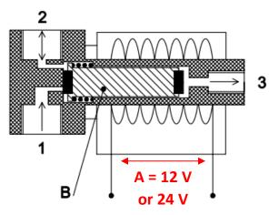
By energizing Solenoid A, plunger B is lifted and connection 1 to 2 is effected. Connection 3 will be closed.
