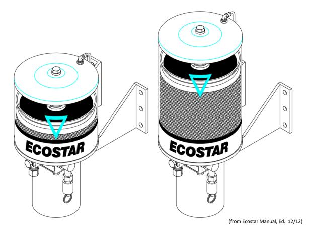
PVP model with support piston at maximum level, 4L (7" tall reservoir) and 6.5L (11" tall reservoir)
